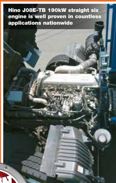
Hino J08E-TB 190kW straight six engine is well proven in countless applications nationwide
